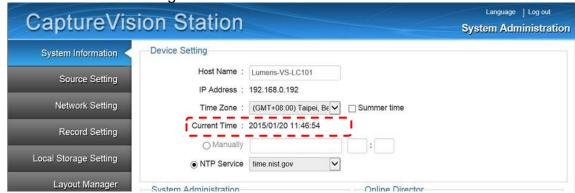
Confirm the time to be correct. If time modification is required, use the manual setting or select other NTP servers.
